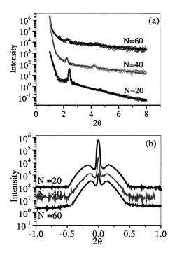
FIG. 2. (a) LAXRD specular spectra taken on a series of superlattices [Fe (3 nm)/Cr (1.2 nm)]<sub>N</sub> with N=20, 40, 60, grown on top of a 100-nm-thick Nb buffer layer. Lines are fits using the SUPREX refinement program; (b) LAXRD rocking curves from the same samples. Spectra are offset for clarity.
