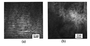
FIG. 3. Cr mapping taken on  $[Fe (3 \text{ nm})/Cr (1.2 \text{ nm})]_{60}$  (grown on Nb), (a) on the first 25 bilayers and (b) the last 25 bilayers.
