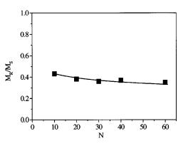
FIG. 6. Remnant magnetization  $(M_R)$  normalized by the saturation magnetization  $(M_S)$  as a function of the number of bilayers (N). Line is a guide for the eyes.
