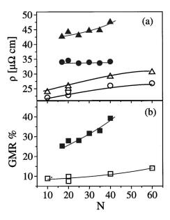
FIG. 8. (a) CPP resistivity  $\rho_{AP}$  ( $\blacktriangle$ ) of [Fe (3 nm)/Cr (1.2 nm)]<sub>N</sub>, CPP  $\rho_P$  ( $\bigcirc$ ), CIP  $\rho_{AP}$  ( $\triangle$ ), and CIP  $\rho_P$  ( $\bigcirc$ ) as a function of N. (b) GMR ratio measured in the CPP ( $\blacksquare$ ) and CIP ( $\Box$ ) configuration as a function of the number of bilayers.
