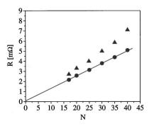
FIG. 7. Perpendicular resistance at 2 K of a series of  $[Fe (3 \text{ nm})/Cr (1.2 \text{ nm})]_N$  measured at zero field (squares) and at saturation (triangles). The solid line is a linear fit. Absolute error bars for each sample are about 15% of the measured resistance.
